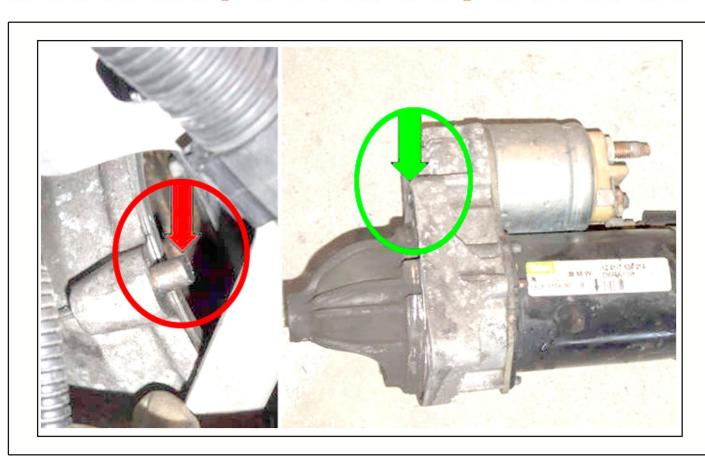
These units have a dowel which is located between the starter motor and gearbox. This allows for the unit to be aligned in the correct position. When removing the old starter motor please make sure the dowel either comes out with the old unit or removed from the gearbox and refitted to the new starter motor. If you fail to do this the unit will not align properly and will cause the unit to be very noisy or fail prematurely. If you don't follow this warning your warranty maybe void.
